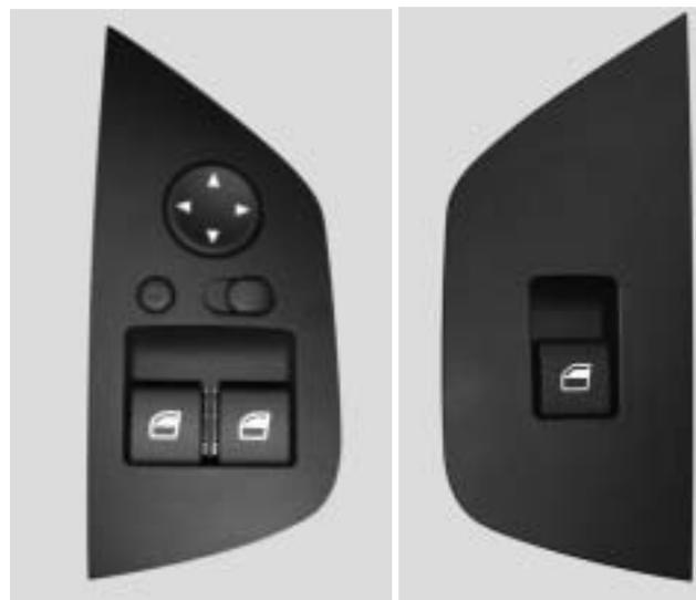
The power-window switches are integrated in the arm rests of the door trim panels. The driver's-side power-window switch unit also incorporates a switch for the passenger-side window, the buttons for the door mirrors and the mirror folding button.
